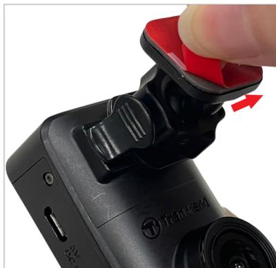
4. Turn the adjustment knob anticlockwise to loosen, and then adjust the DrivePro's position.
